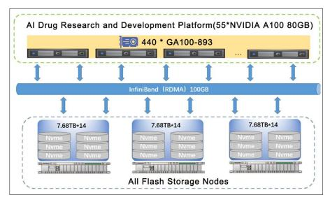
In this project, 3 storage servers are used, each equipped with 14\*7.68TB NVMe disks as the unified shared storage system of the AI drug research and development platform, supporting the front-end 55 NVIDIA A100 80GB computing servers with a total of 440 GPU cards with model GA100-893 for deep training and new drug development.
