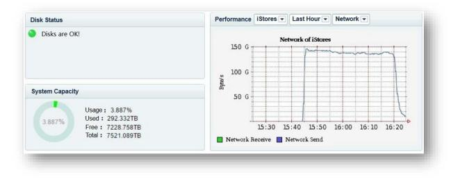
Customer on-site 7.5PB LeoFS system, consists of 102 nodes of 4U 24-bay storage servers, with totally 1,880 drives of 4TB SATA HDDs. Dual 10GbE network is used and provides an aggregated I/O close to 150GB/s. Average single drive write 75MB/s.
